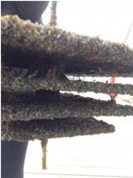
A provincial substrate sampler encrusted in a half-inch thickness of zebra mussels on all surfaces. This sampler was removed from Gimli Harbour in September, 2015, after being left in the water for three consecutive months. (Photo: Manitoba Conservation and Water Stewardship)
