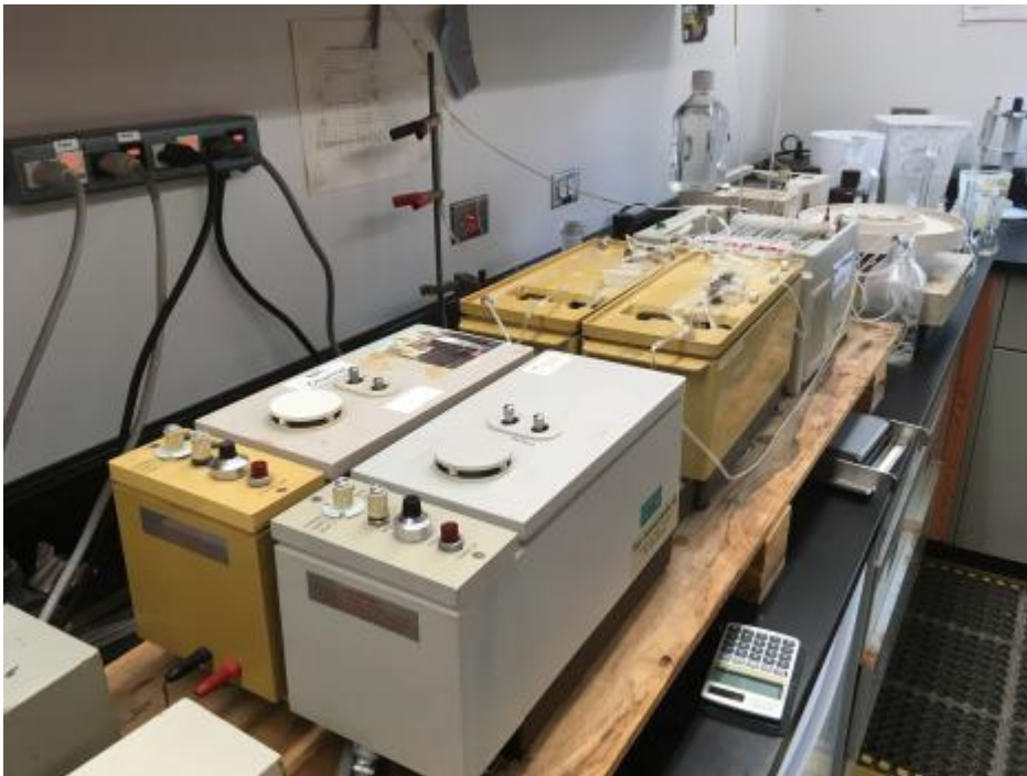
IISD-ELA's on-site chemistry lab processes 20 to 30 water samples every week. Ten different analyses are conducted in house; six more are done at the University of Alberta. This auto-analyzer runs collected samples to measure phosphorus levels.
