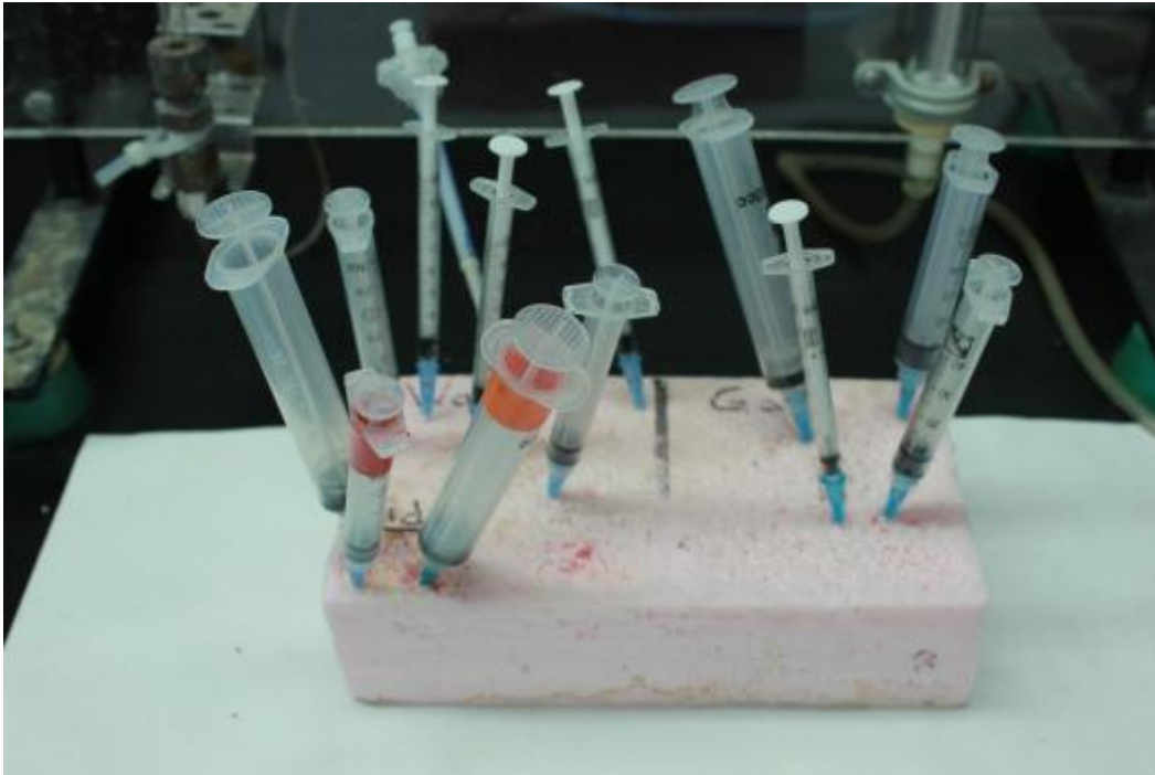
Syringes, part of a homemade gas chromatograph set-up that measures carbon dioxide levels
